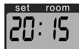
F: When the 4-digit stops blinking, the setting has been locked to the indicated value.
